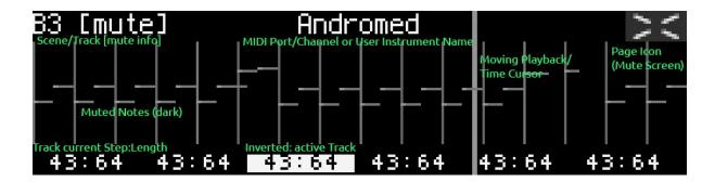
Here the MUTE screen of Track 3, Scene B is displayed, which is currently muted and mapped to user instrument "Andromed" and the current playback position of this clip is step 43 of 64. The sequencer is running and the time cursor is almost three quarters through the clip. The six tracks can be muted and unmuted by pushing the upper-row keys in this screen.
