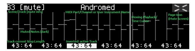
Here the MUTE screen of Track 3, Scene B is displayed, which is currently muted and mapped to user instrument "Andromed" and the current playback position of this clip is step 43 of 64. The sequencer is running, the time cursor is about three quarters "through the sequence" and the lower six tracks are available for muting and unmuting by pushing the first row of keys.
