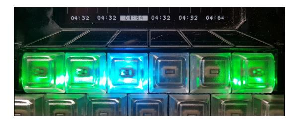
In the often-used MUTE screen, pushing one of the six keys mutes or unmutes one of the six tracks (unmuted tracks are also illuminated in green). The currently active track is indicated with a blue backlit key. Therefore, if a track is both active and unmuted, this leads to a cyan color mix (green and blue); see track three in the above picture.
