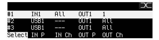
MIDI packets can also be forwarded to (or sent from) a virtual USB port (when connecting LoopA to Windows 10 or Mac OS via USB. Four independent MIDI USB devices are added and could redirect MIDI traffic around a studio.
