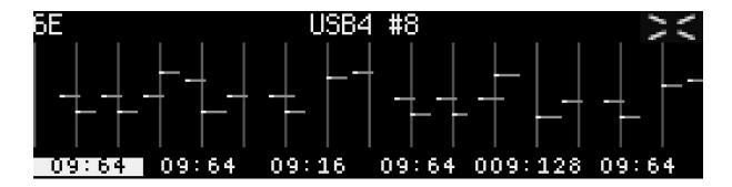
The above screenshot displays a 64-step sequence with stored note data track 6, scene "E", shortened to "6E". The output port is USB4 MIDI port, channel 8.
