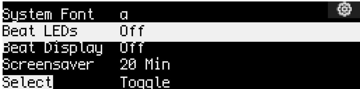
In the setup screen, use the lower-left SELECT knob to scroll through the configuration items and to select an active item. Use the upper-row keys below the OLED to select parameter values and either simply "toggle" them by pushing the respective upper-row key (e.g. toggle Beat LEDs "on" or "off"), or if a value is selected, use the lower-right VALUE knob to change settings (e.g. change the OLED Screensaver activation time).
