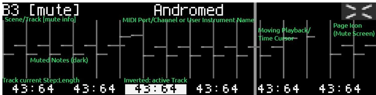
Here the MUTE screen of Track 3, Scene B is displayed, which is currently muted and mapped to user instrument “Andromed” and the current playback position of this clip is step 43 of 64. The sequencer is running, the time cursor is about three quarters “through the sequence” and the lower six tracks are available for muting and unmuteing by pushing the first row of keys.
