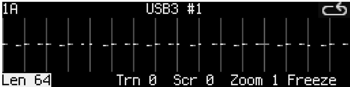
The active clip is displayed in the top-left corner (e.g. 1A corresponding to track 1, scene A). The following operations are available on the top row of keys:
