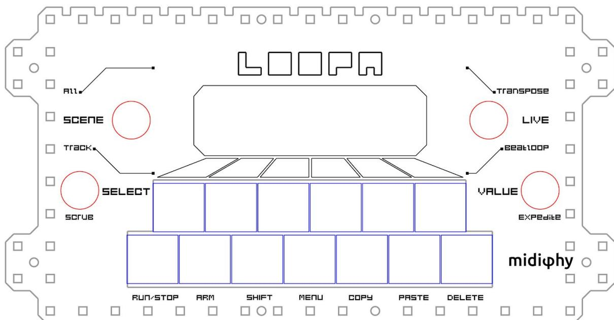
The user interface consists of a 256x64 pixel, 16 grayscale-level OLED, four knobs (red) with status indication LEDs around the upper knobs and thirteen keys (blue) organized in two rows, the upper keys are often directly associated with onscreen actions of the currently active screen and the lower keys operate basic functions (e.g. sequencer RUN/STOP) that are available from every screen.
