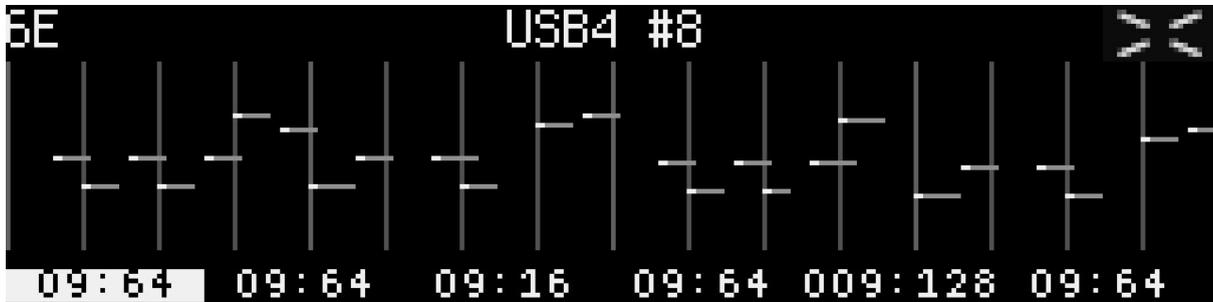
The above screenshot displays a 64-step sequence with stored note data track 6, scene "E", shortened to "6E". The output port is USB4 MIDI port, channel 8.
