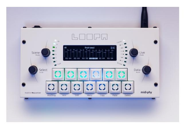
The user interface consists of a 256x64 pixel, 16 grayscale-level OLED, four black knobs with status indication LEDs around the upper knobs and thirteen mechanical keyswitches organized in two rows. The upper keys are typically associated with onscreen actions of the currently active screen and the lower keys operate basic functions (e.g. sequencer RUN/STOP) that are available from every screen.
