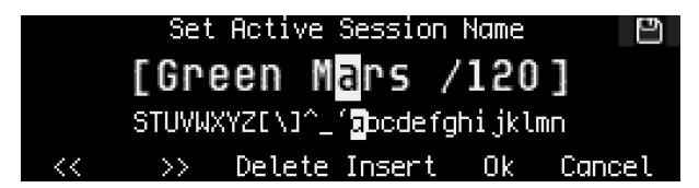
Move the cursor with the "<<" or ">>" commands or by turning the SELECT encoder. Change a character at the cursor position by turning the VALUE knob. Delete and insert characters with the respective keys and finally use "Ok" or "Cancel" to set a new session name or to revert to the old name.
