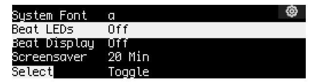
In the SETUP screen, use the lower-left SELECT knob to scroll through the configuration items and to select an active item. Use the upper-row keys below the OLED to select parameter values and either "toggle" the the value by pushing the respective upper-row key (e.g. toggle Beat LEDs "on" or "off"), or if a value is selected, use the lower-right DATA knob to change settings (e.g. change the OLED Screensaver activation time).
