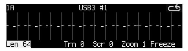
The active clip is displayed in the top-left corner (e.g. 1A corresponding to track 1, scene A). The following operations are available on the upper-row keys and (apart from Freeze) modified with the DATA knob:
