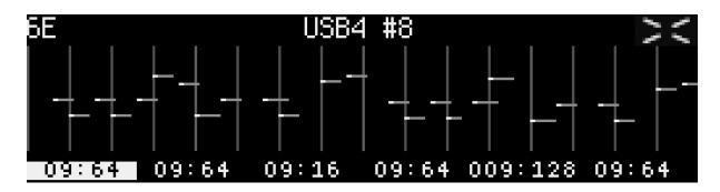
The above screenshot displays a 64-step sequence with stored note data on track 6, scene "E", shortened to "6E". The output port is USB4 MIDI port, channel 8.
