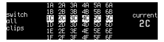
The currently active "scene-switching mode" is displayed on the left. The mode can be changed by quickly pressing and releasing the SCENE knob button and is indicated by a front-panel LED.
