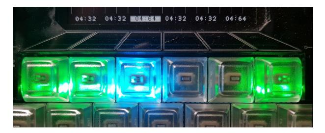
In this example displaying the MUTE states, pushing one of the six upper keys mutes or unmutes one of the six tracks. In this picture, unmuted tracks are illuminated in green but this behavior may be inverted in the SETUP screen if muted tracks should have an "active" LED state. The currently active track is indicated with a blue backlit key. Therefore, if a track is both active and unmuted, this leads to a cyan color mix (green and blue); see track three in the above picture.
